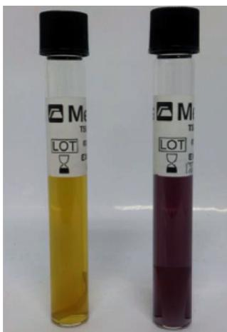
The tube on the left indicates survival of the BI (acid produced) and that on the right is sterilized (color is unchanged).
